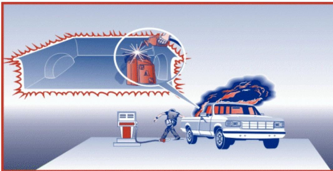
**Fire Hazard:** Filling gas can in pickup truck with plastic bed liner.
