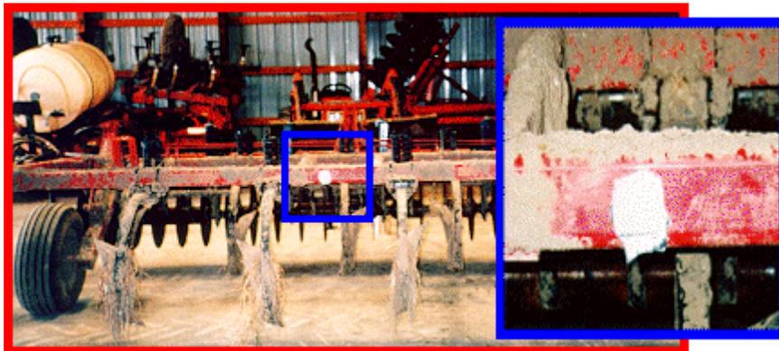
**Ignition Hazard: Drilling, cutting or welding a sealed frame on agricultural equipment can result in a gas explosion.**
